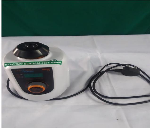
The Vortex Mixer is used to agitate samples and promote homogenization of samples in test tubes
