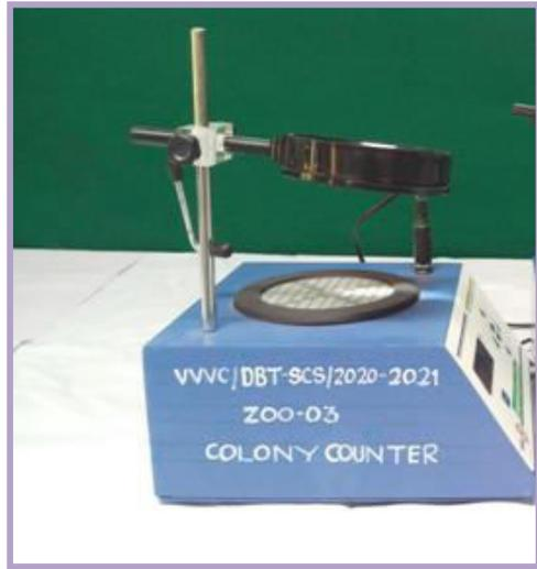
Colony counter is used to count the number of colonies of bacteris in sample of food (CFU/mg) or water (CFU/ml)
