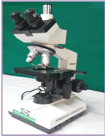
A trinocular microscope is used to take pictures and also record videos of the specimens to be observed. It has two eyepieces like a binocular microscope and an additional third eye tube for connecting a microscope camera
