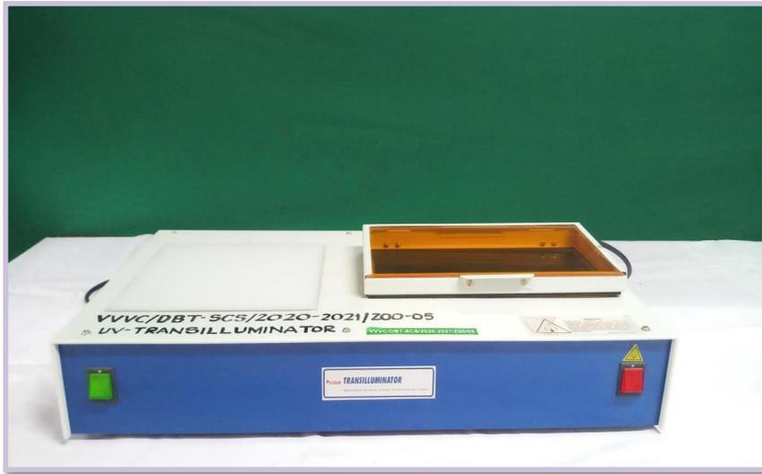
This instrument is used in molecular biology to visualize the proteins, DNA or RNA bands separated using Gel Electrophoresis
