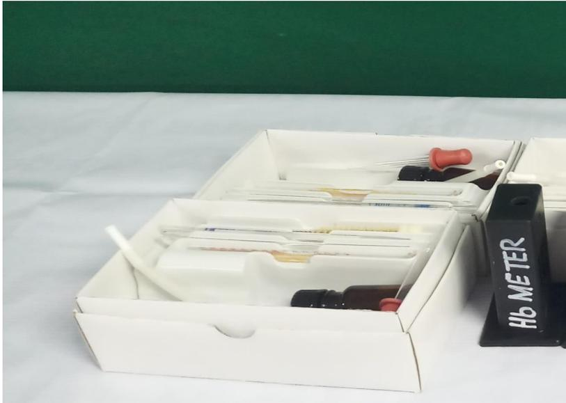
It is an instrument used to determine the quantity of haemoglobin in the blood. It is based on comparison of the colour of the tested blood, which is treated with hydrochloric acid, with the colour of standards
