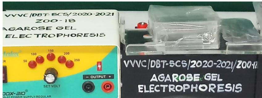
Agarose gel electrophoresis is a general term that is used for the separation of charged particles (ions), the DNA under the influence of an electric field.
