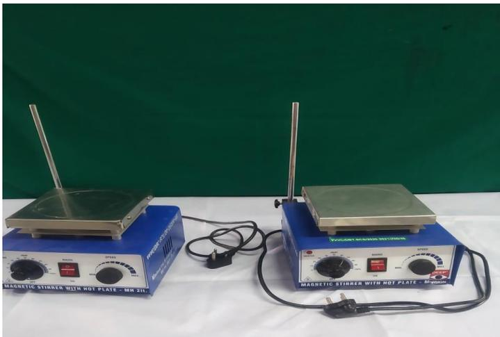
A hot plate magnetic stirrer is used for mixing and heating aqueous solutions simultaneously to speed up the reaction and dissolve the solute in the solvent.
