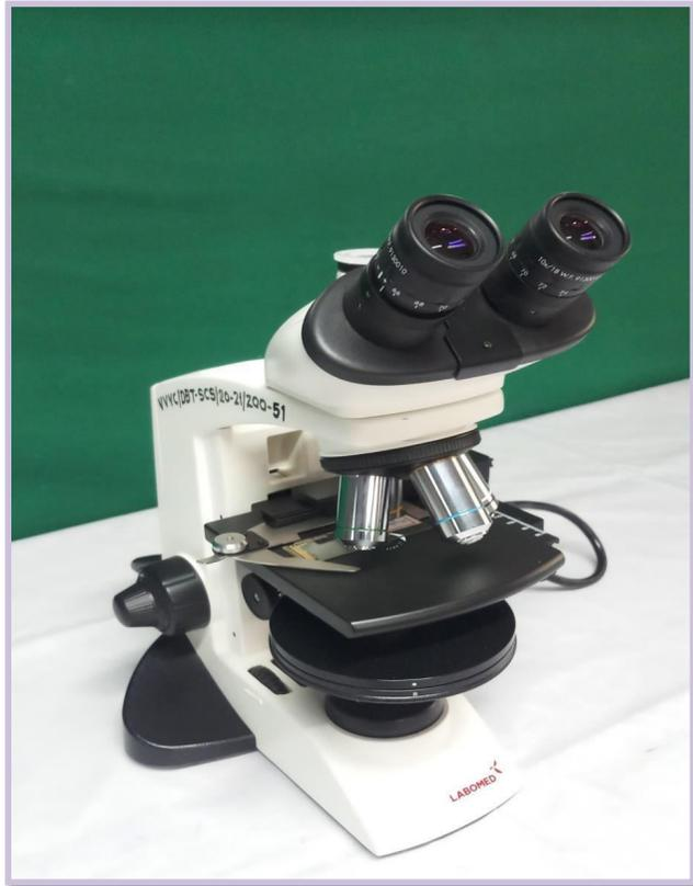
Phase contrast microscope is used to observe living cells and their motility. It provide high-contrast, high-resolution images.
