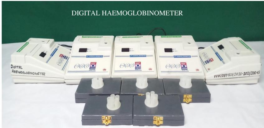
The Digital Hemoglobinometer is a portable device used to measure the concentration of haemoglobin in blood. The measurement of haemoglobin is important to diagnose anaemia or high haemoglobin levels in the assessment of changes before and after operations or blood transfusion.
