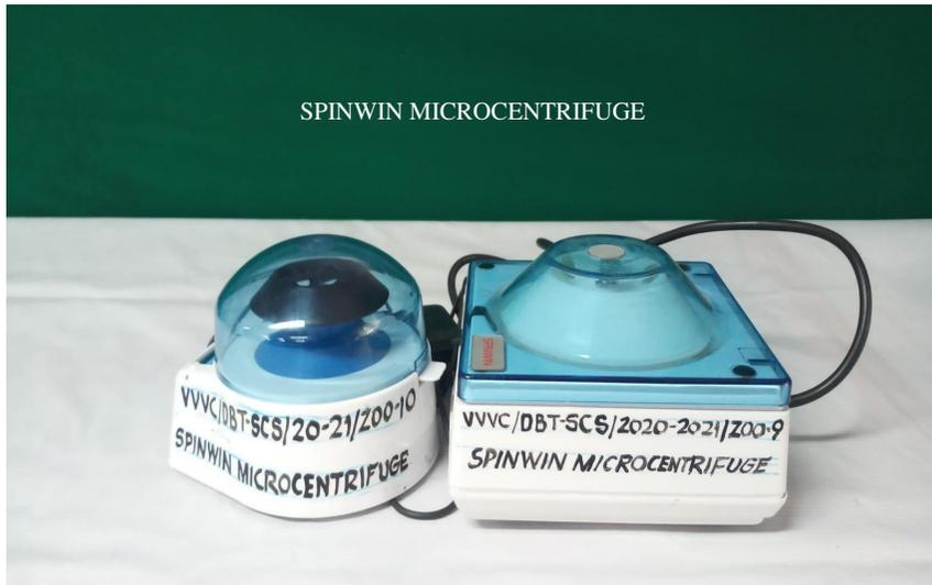
Spinwin micro centrifuge helps to accommodate PCR tubes and micro centrifuges for continuous separations of components in a sample with safety lid lock and lid drop protection.
