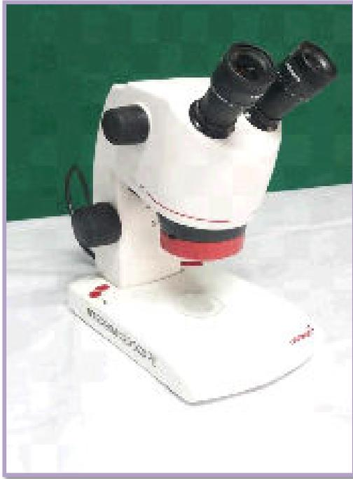
Stereomicroscope is used to examine the opaque specimens and provide 3D view of the insects or any part of the plant that are normally visible to the naked eye.
