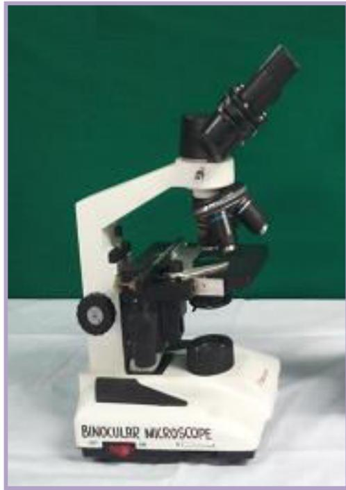
Binocular microscopes are used to carry out the microscopic analysis of blood cells and to detect abnormal changes in cell or tissues. It reduces the eye strain caused by the monocular microscopes when observe the cells for long periods of time.
